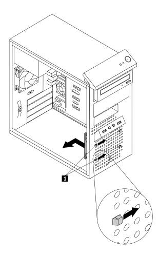
Figure 41. Removing the front fan assembly
